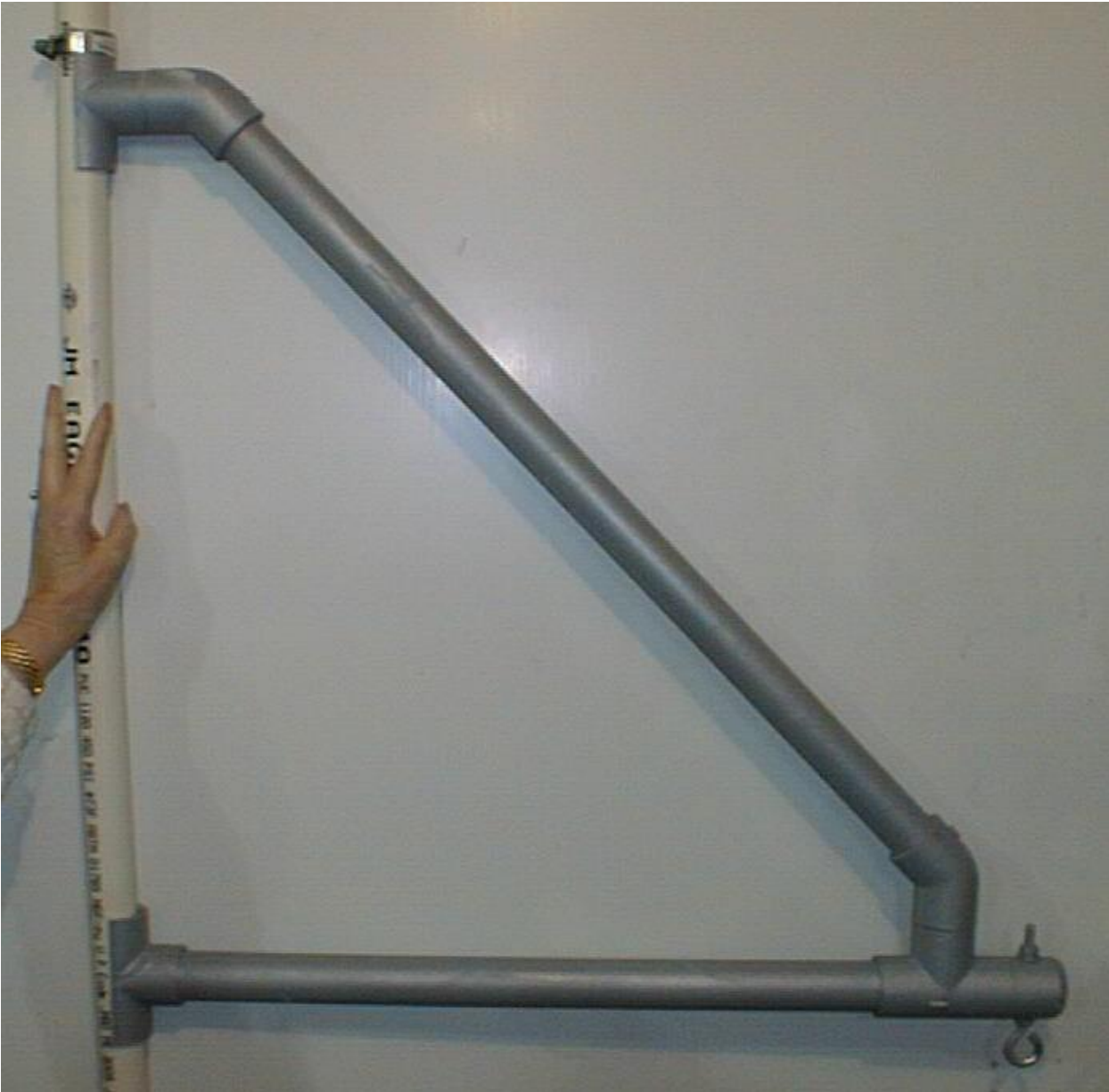
[Fig 1] Completed assembly with coat of gray paint. White vertical member on left is for demonstration only. This mount would be attached to the vertical leg of a Rohn Tower using four stainless steel hose clamps.
